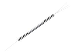
The FC Series 1x3 Compact Fiberoptic Splitter is based on Agiltron's fused biconical taper technology and compact packaging structure. It features superior uniformity, low excess, and very low polarization sensitivity. The device is ideal for splitting or combining light with exceptional performance over a wide wavelength range.
